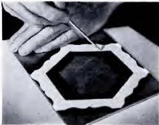
Above, brass is painted with India ink and the outline of the trivet frame is scribed on the brass, using a cardboard template. Holes for the finials are center-punched, drilled and then tapped, as below
